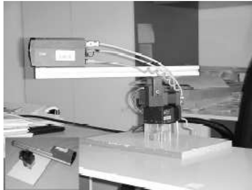
Figure 1.8: 3D depth measurement sensor using a camera mounted on a rotating robot arm. Courtesy of Peer P. from the University of Ljubljana
