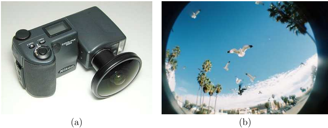
Figure 1.6: Fisheye lenses. (a) Nikon Fisheye Converter FC-E8 mounted on a Coolpix 990. (b) Image captured using fisheye optics.
