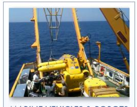
**MARINE VEHICLES & ROBOTS** 3 marine vehicles were used during the cruise: THETIS, a **Human Operated Vehicle** (HOV); MAXROVER, a remotely operated vehicle (ROV); and GIRONA500 an Autonomous Underwater Vehicle (AUV). THETIS and MAXROV are vehicles owned by the HCMR. GIRONA500 is an AUV designed and developped by GIRONA500AU the University of Girona.
