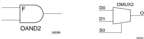
Figure 20: AND & MUX Symbols in XC4000X IOB
