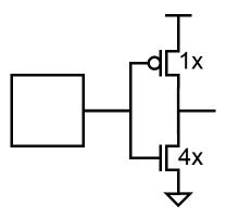
Since the gate dimensions are weird, and because the input levels might not turn the transistor fully on or off, this inverter is usually small. This means to drive a long wire to the core of the chip will take some level of buffering.
