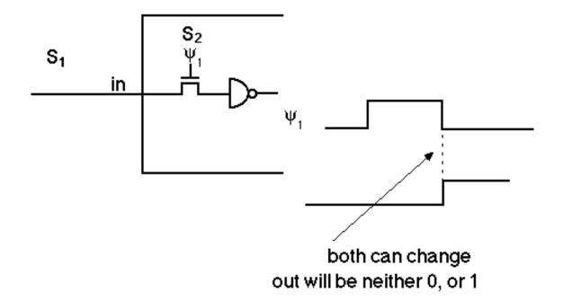
A simple dynamic latch could get an output that would be between 0 and 1.
