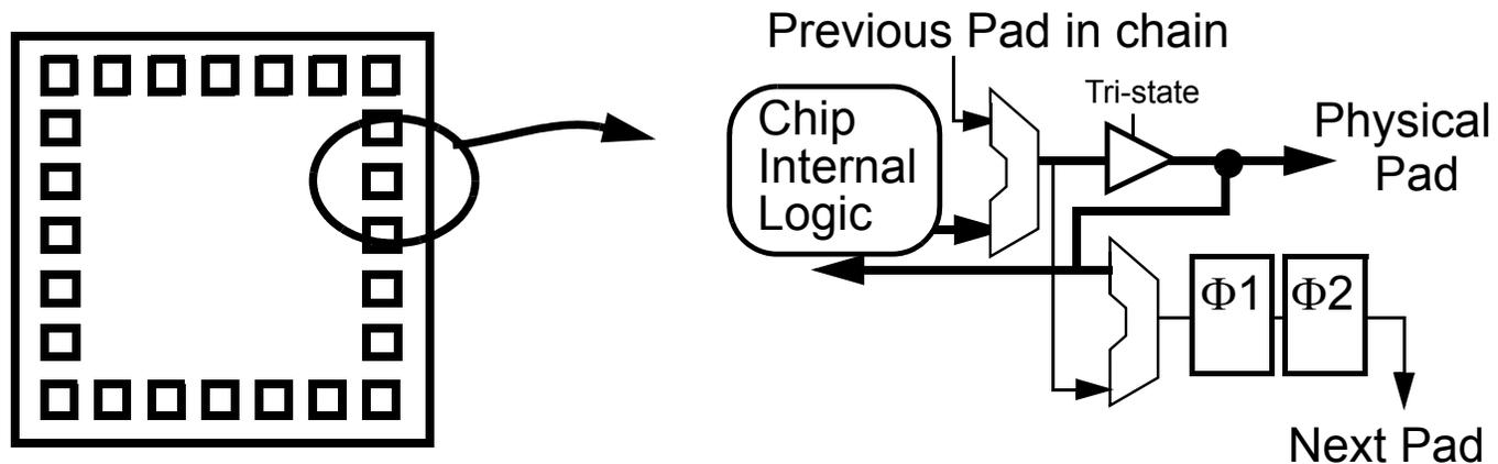
Using ability to make every pin either an input or output, the tester drives a value on a pin, and then checks the input pins of the other chips that should be connected to this chip. If they don't see the same value, the 'board' is not working correctly (could be solder connections, or a broken via in the board)
