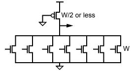
• But static load circuits have the nMOS problems: – DC power and ratio rules For a 4:1 current ratio, the nMOS width  $(w_n)$  must be twice  $w_p$
