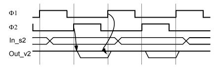
Could also choose to flip  $\Phi$ 1 and  $\Phi$ 2, and have the gate evaluate on  $\Phi$ 1
