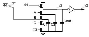
You need to watch for **charge-sharing** in the series devices. If A and B rise, but C remains low, then C1 and C2 will share charge with Cout. Since A and B could have been low during precharge, C1 and C2 might be low, and Cout better be much larger than C1+C2. If that is not the case, you can add more precharge transistors, as shown in grey.
