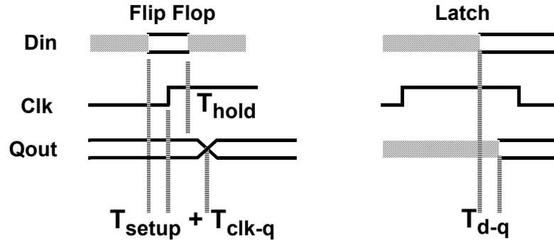
Flip-flop delays the slowest signal by the setup + clk-q delay
