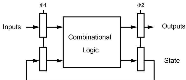
This is a Moore machine, since both the state and the outputs are registered (you could consider the outputs to be more state bits). But since you call only some of the outputs state bits, you can implement a Mealy state transition diagram this way.
