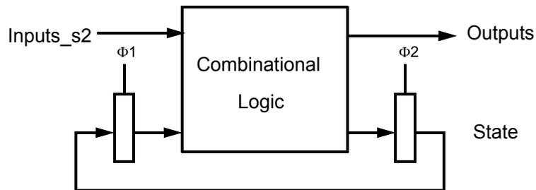
This is a Mealy machine, since the outputs are a direct function of the inputs. Note that the inputs and the state inputs to the combination logic need to have the same timing type ( $\_s2$  in this case).
