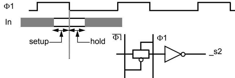
Signal must settle before  $\Phi 1$  falls, and not change for some time after  $\Phi 1$  falling, even for a skewed  $\Phi 1$  (this is usually called the setup and hold times of the latch)
