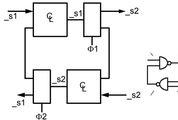
No static feedback in the combination logic is allowed either. This makes the system not sensitive to logic glitches.
