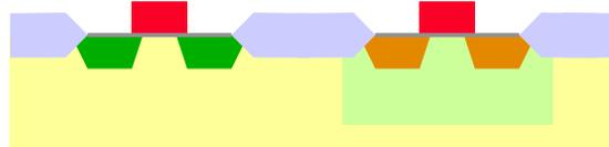
5. Coat the top of the poly and diffusion with metal to reduce resistance. (silicide)
