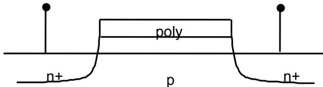
Diffusion is made by adding (diffusing) impurities into the silicon
