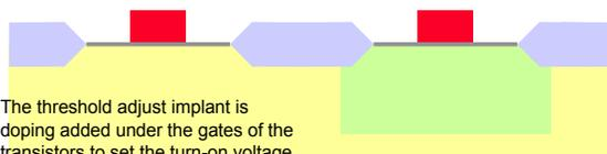
The threshold adjust implant is doping added under the gates of the transistors to set the turn-on voltage of the transistors (threshold voltage) to the correct value.
