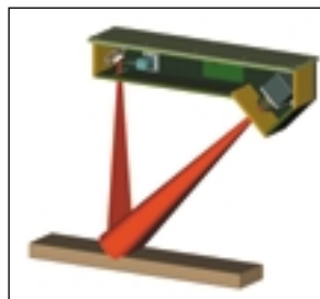
Optical principle of INO 's 3D laser profiling sensor.
