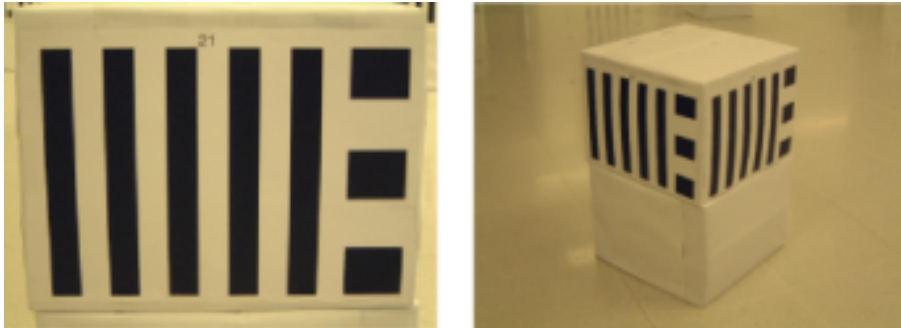
Figure 6.3: Left : Landmark label 21 (code = 10101 = 21). Right : One of the boxes with multiple landmark labels
