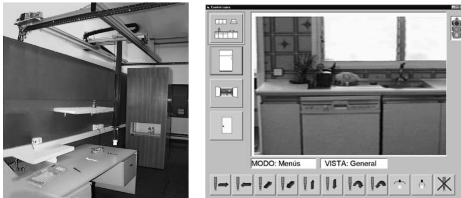
Figure 2: The left image shows a first prototype of the robotized kitchen in the lab environment. The right image is a view of the kitchen interface.
