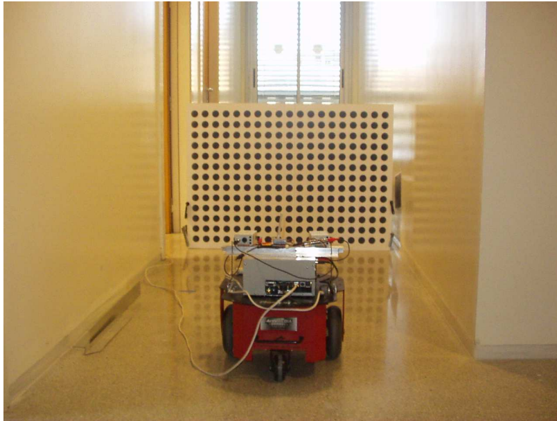
Figure 6.3: Stereo camera over a mobile robot.
