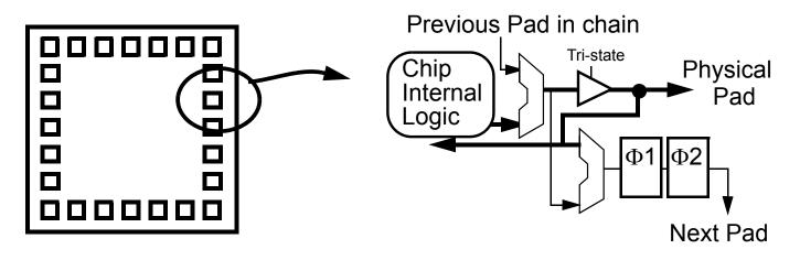
Using ability to make every pin either an input or output, the tester drives a value on a pin, and then checks the input pins of the other chips that should be connected to this chip. If they don't see the same value, the 'board' is not working correctly (could be solder connections, or a broken via in the board)
