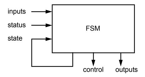
It is usually an FSM since some operations that the chip performs take multiple clock cycles, and the controller must know where it is in the instruction.
