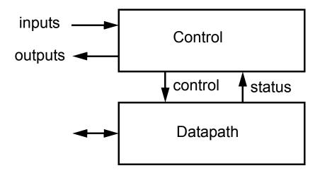
When the datapath is pipelined (multiple parts of operations in progress simultaneously), the control keeps track of the status of all of the pieces.
