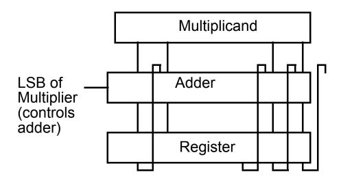
This hardware generates a 2n bit result, so you need to catch the bits that shift off the end of the register. If you only wanted to generate an n bit result, then it would be better to shift the multiplicand to the left.<sup>1</sup>
