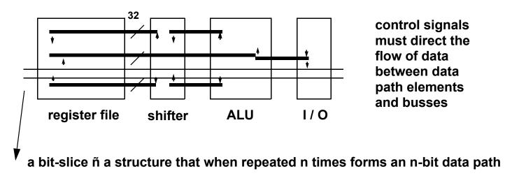
• Problem is that all cells must have the same height -- means you need to estimate which cell is the tallest, and use that to set bit pitch.
