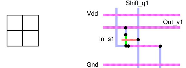
Cells don't use Vdd, Gnd, but need to route them for the other cells. The shift cells should not be mirrored (all nMOS so there is no need), but can fit in with a mirrored datapath (just change Vdd Gnd names)
