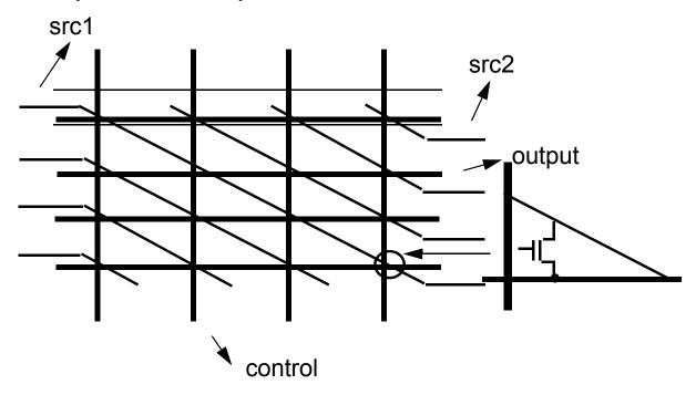
Inputs are driven from both sides, and then run diagonally through the array. Control runs vertically, and the output runs horizontally.
