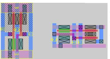
Notice the wide M2 power lines on the left cell. Also notice that the M1 wires generally can't run on top of stuff
