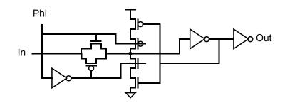
Notice this latch requires no ratioing of transistors or capacitance.
