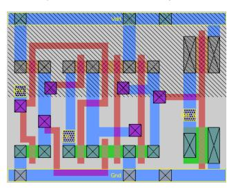
This layout has been hacked some from simply laying out poly. But only real cleverness is the merging of the TG diffusion with the tristate inverter, and the routing of the clock lines to this section. And even in this section it is still poly mostly vertical.
