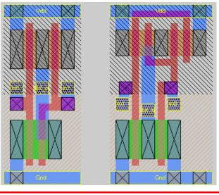
There are well and substrate contacts under the supply lines (on top and bottom of cell)
