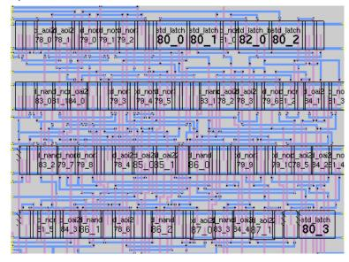
Generally macros have more structured wires than standard cells, so you need to use a little different implementation style for the cells. For structured wires, the cells contain the wires and snap together.
