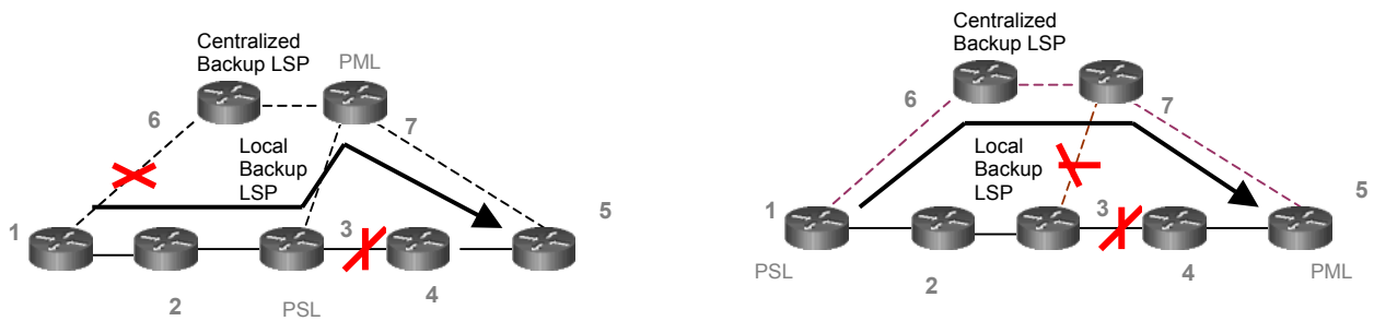
Figures 22 (a), (b) : Multilevel protection application.
